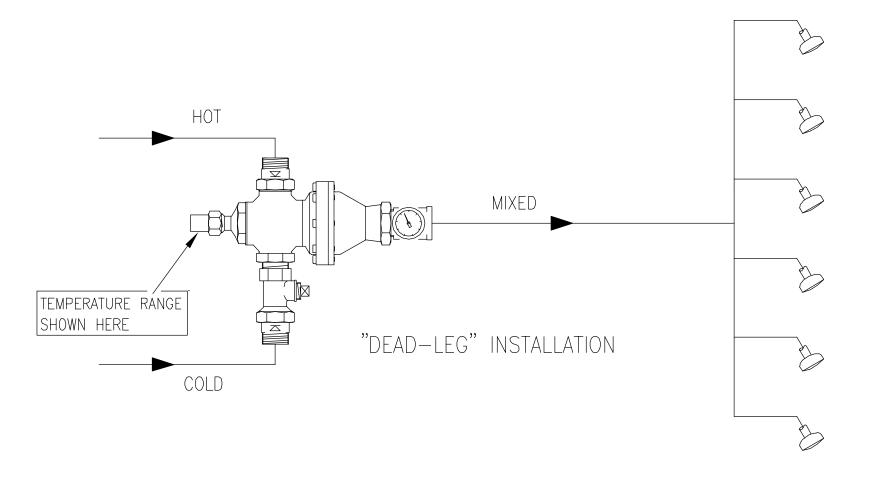
NOTE: BEFORE INSTALLATION, CHECK THAT THE TEMPERATURE ADJUSTMENT RANGE IS SUITABLE FOR THE INTENDED USE. THE TEMPERATURE RANGE IS SHOWN ON THE LOCKSHIELD NUT AT THE ADJUSTING SCREW. (SEE ABOVE)
